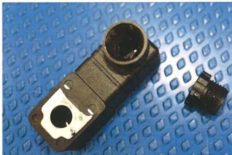
IPX5 Post Test Observation photos for Solenoid coils
