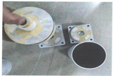
The IP test procedure is based on IEC 60529(Degrees of Protection provided by enclosures IP Code). After the completion of each test sample was visually inspected.
