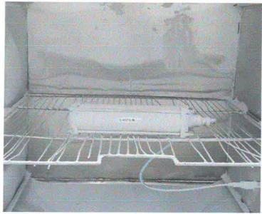
The sample during protection against water test was seen as follows:
